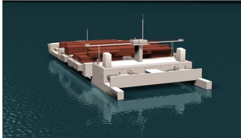
Fig. 1: The TSL carries barges athwart ship on 3 cargo platforms. Two ship-borne tugs in dry berth at the stern facilitate barge handling.
